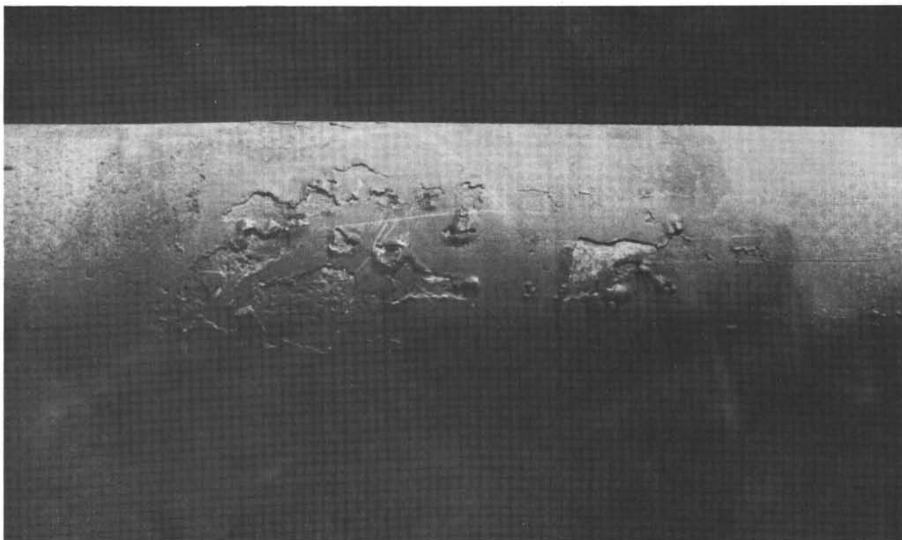
EXFOLIATION OF ALUMINUM DRILL PIPE FIGURE 11
