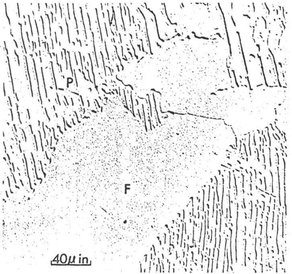
X-60 STEEL as received. Ferrite area is marked "F" and pearlite area, "P." The appearance of X-52 is similar but the width of the carbide platelets in the pearlite and the ferrite grain size are about twice as big in X-52 as in X-60. Fig. 16.
