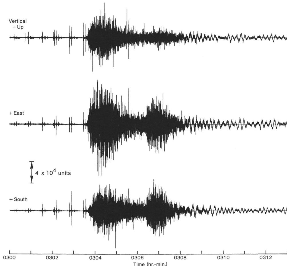
Figure 1. The 26 May 1983 Japan earthquake recorded (unfiltered) by the OSS IV geophones. The spiky arrivals before the earthquake are SUS charge signals.
