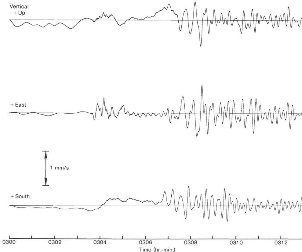
Figure 3. The Japan earthquake recording filtered to be flat to velocity from 64 s to 4.5 Hz. This trace emphasizes the long-period arrivals.
