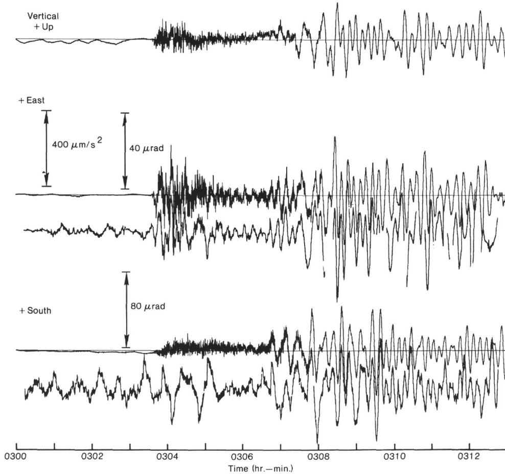
Figure 5. A comparison of the OSS IV tilt meter and geophone traces for the Japan earthquake of 26 May 1983. The geophone traces are filtered to be flat to acceleration from 64 s to 4.5 Hz. The OSS IV tilt meter records are shown below the two horizontal geophone traces. Note that the + south tilt meter is plotted at half the vertical scale of the other sensors.
