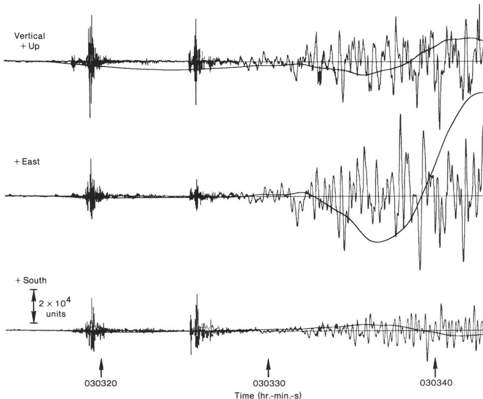
Figure 2. The Japan earthquake early wave arrivals on an expanded time scale. The high-frequency trace is unfiltered; the smooth trace is low-pass filtered (three poles) at 16-s periods. The filtered data are plotted on a vertical scale  $50\times$  that of the unfiltered data. The sharp arrivals in front are from an SUS charge. Note the emergent onset of the  $P_0$  wave ahead of the impulsive long-period P-wave.
