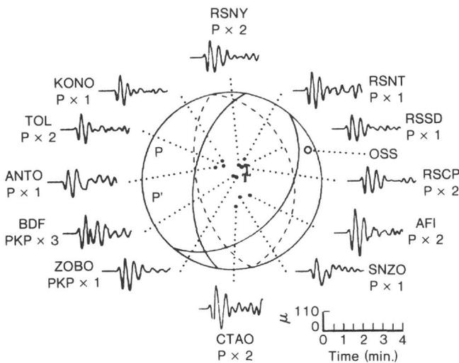
Figure 4. Focal mechanism of the 26 May 1983 Japan earthquake as published in the NEIS monthly listing, together with the OSS IV first motion. Acronyms are seismic station names. The focal mechanism is consistent with thrust faulting.
