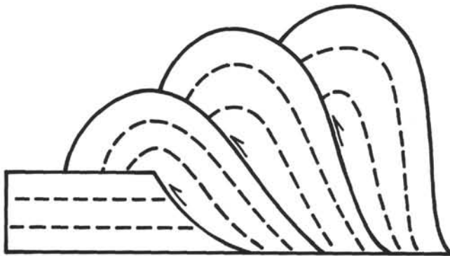
Figure 5. The imbricate underthrust accretionary model of Seely et al. (1974). Sediments (flat-lying segment to left) are progressively scraped off the underlying ocean crust and incorporated into the accretionary wedge to the right. Insertion of each new wedge into the bottom of the stack elevates and rotates overlying wedges with the result that major boundaries and internal stratigraphy (possibly LDRs) exhibit progressive steepening of dip upslope.
