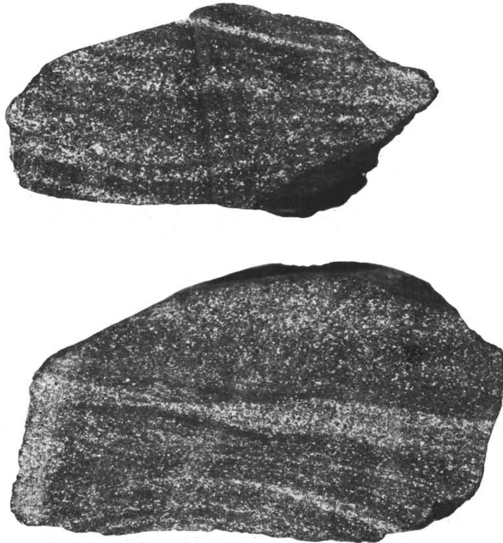
Figure 4. Indurated (palagonitized) bedded tuff, Sample 483B-8-1, 21-28 cm. (See Fig. 1 of plate for photomicrograph of tuff.)
