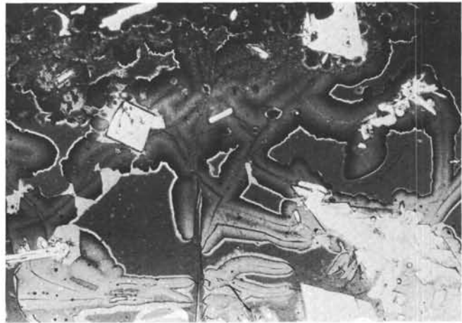
Plate 1. Tephra deposits recovered on Leg 65. 1. Marginally palagonitized shard in center of photomicrograph showing layers of "gel-palagonite" (width of photomicrograph, 2 mm), Sample 483-7-2, 11-16 cm. 2. Fresh sideromelane shards set in nonvolcanic silt and fecal pellets (note angular blocky shape of shards); former palagonite rim of some shards has been removed by grinding (width of photomicrograph, 5 mm), Sample 483-7-2, 11-16 cm. 3. Indurated hyaloclastite consisting of completely altered sideromelane shards set in a nonvolcanic matrix of silt and fine sand. The shards are now represented by light smectite, concentric banding representing successive stages of palagonitization and a dark Ti-rich(?) phase. The large plagioclase crystal (right) has also been marginally dissolved, the void being partially filled by zeolite (width of photomicrograph 5 mm), Sample 483B-8-1, 21-28 cm. 4. Photomicrograph of glass alteration at the base of a massive flow. Dark brown homogeneous areas are sideromelane, grading outward into a colorless "palagonite" rim followed, across a sharp transition, by dark through light-brown "palagonite" (width of photomicrograph, 5 mm), Sample 483B-26-1, 39-40 cm.
