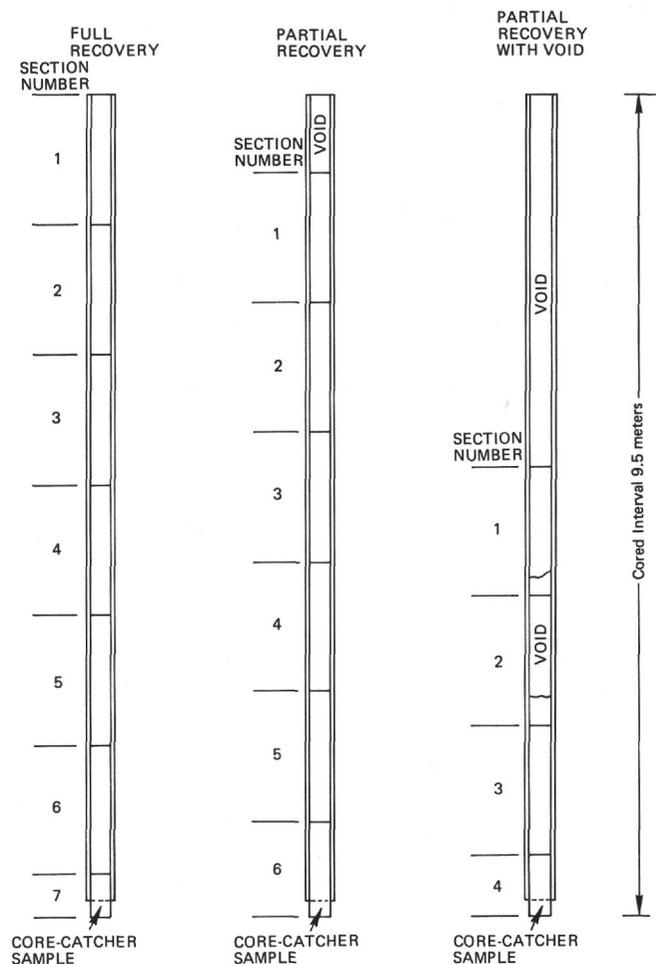
Figure 1. Labeling of sections for various kinds of recovery.
