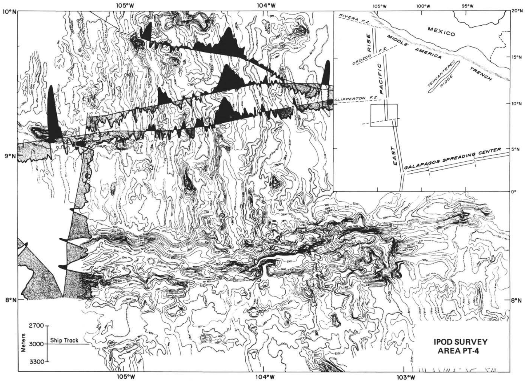
Figure 2. Bathymetry profiles along ship tracks. Base level (ship track) = 3000 meters. Bathymetric contours from Rosendahl (this volume).
