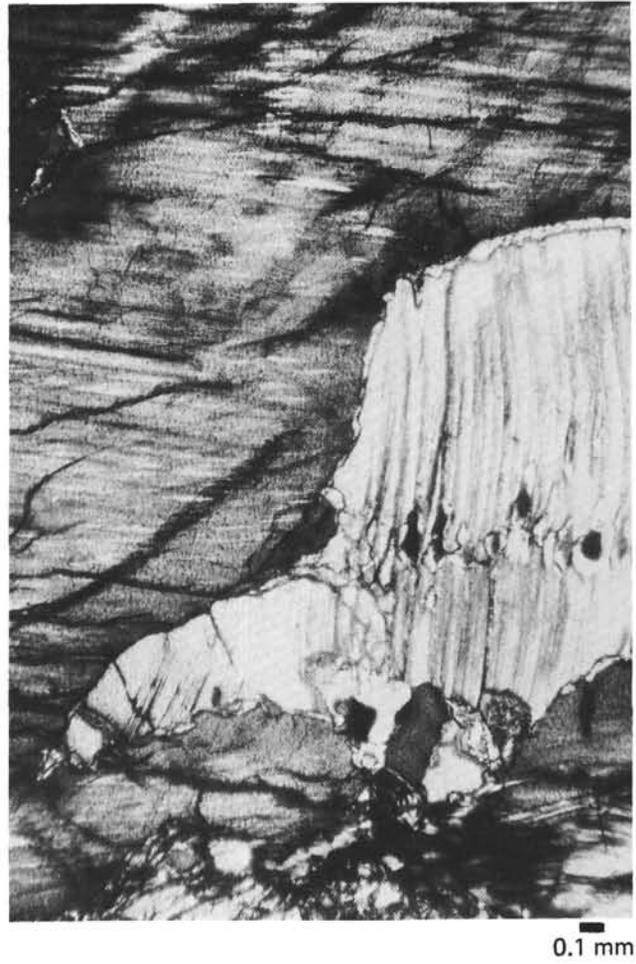
Figure 4. *Photomicrograph of a clinopyroxene porphyroclast (white) associated with an enstatite porphyroclast (gray). Lherzolite, piece 17f; crossed nicols.*
