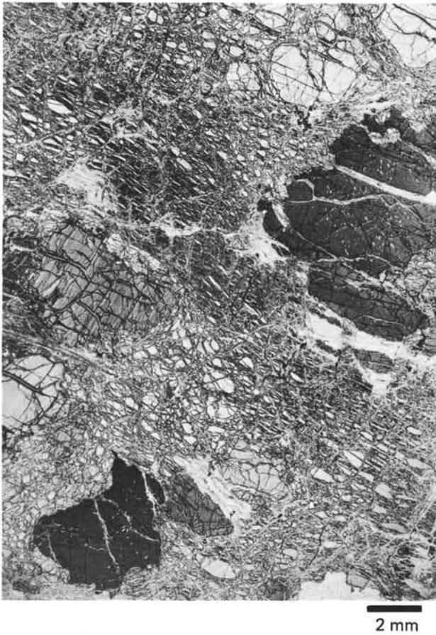
Figure 3. *Photomicrograph of harzburgite, piece 2g, in a thin section cut perpendicular to the foliation whose trace is southwest-northeast on the figure. Elongated enstatite sections contain (100) exsolution lamellae. The principal plane of serpentinization is perpendicular to the trace of the foliation. Crossed nicols.*
