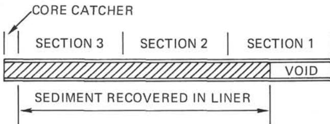
Figure 7. Diagram illustrating convention for placement of sections in a core, and identification of the top of a core.
