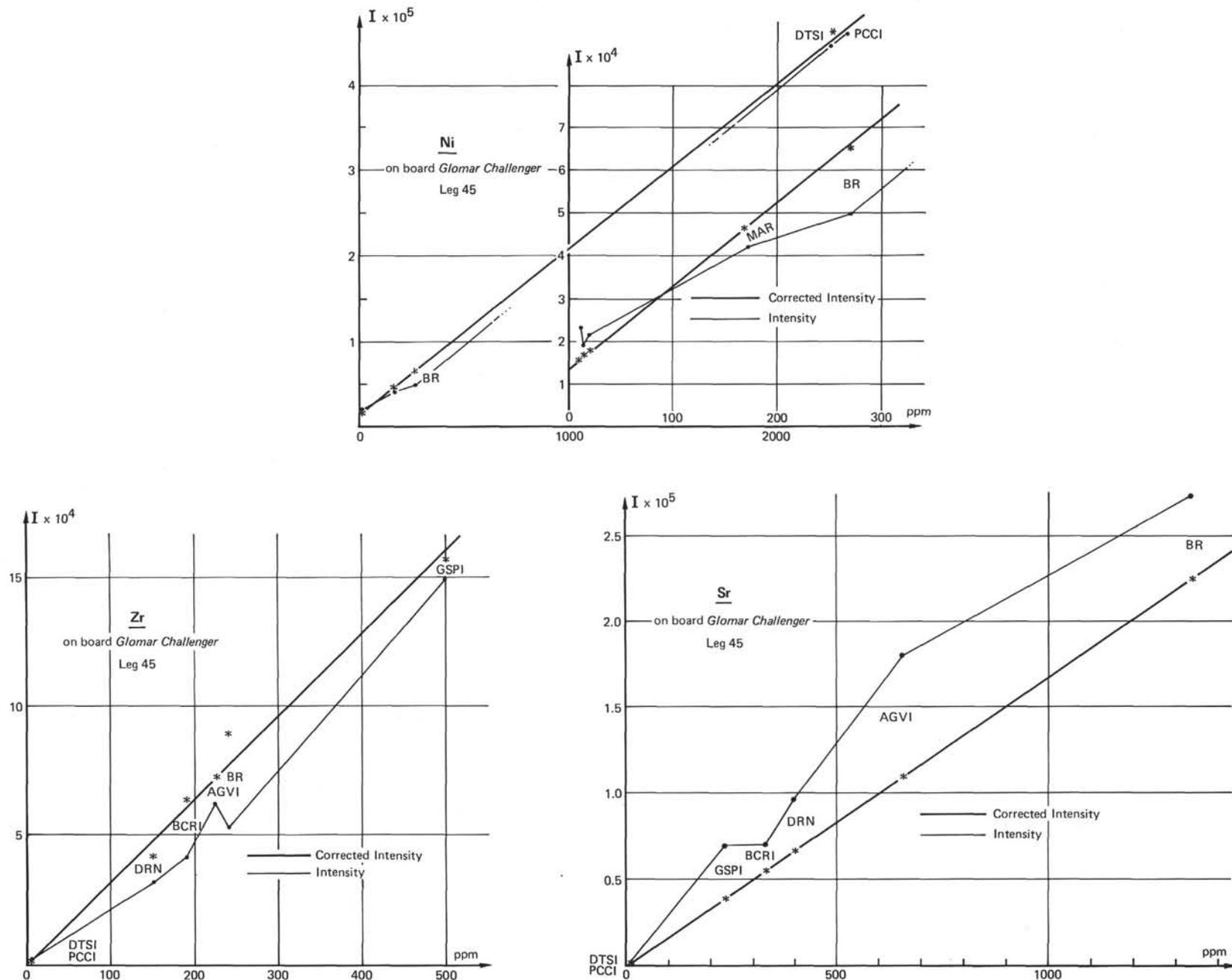
Figure 6. Calibration curves for Ni, Sr, and Zr determined on board ship during Leg 45.
