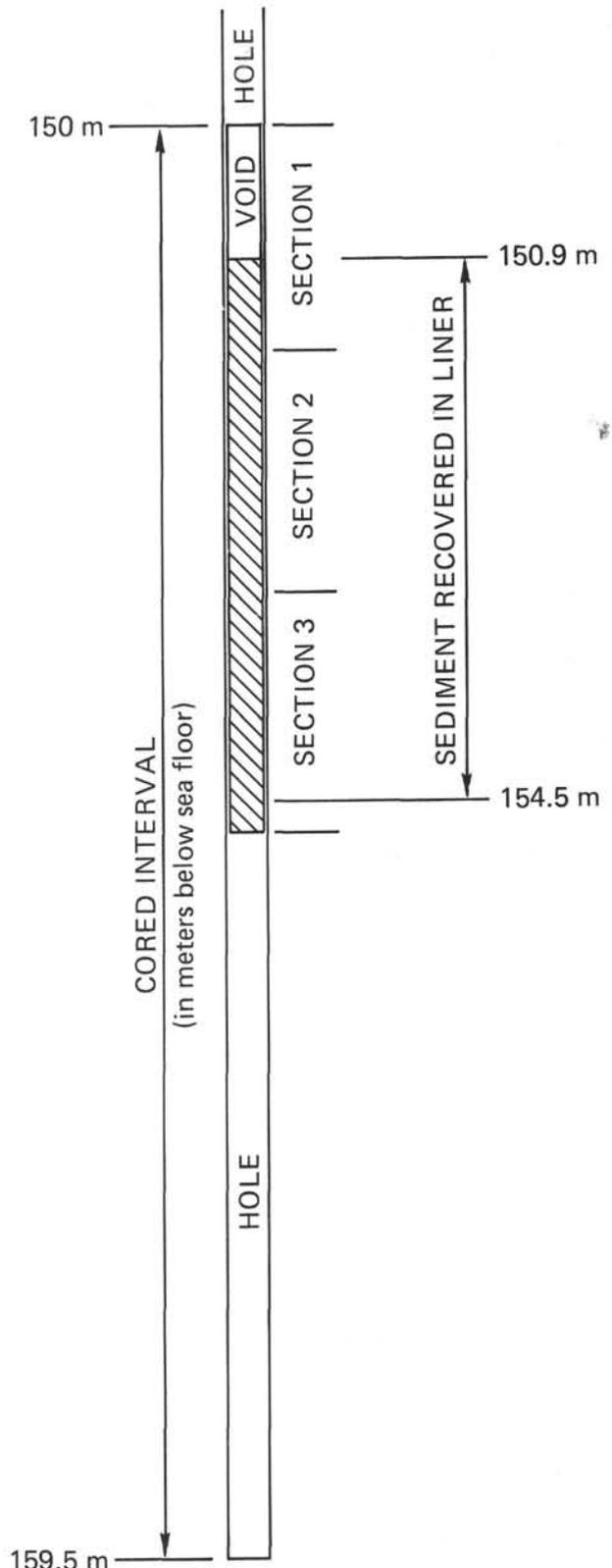
Figure 8. Diagram illustrating convention used on Leg 45 for placement of sections within a 9.5-meter interval.
