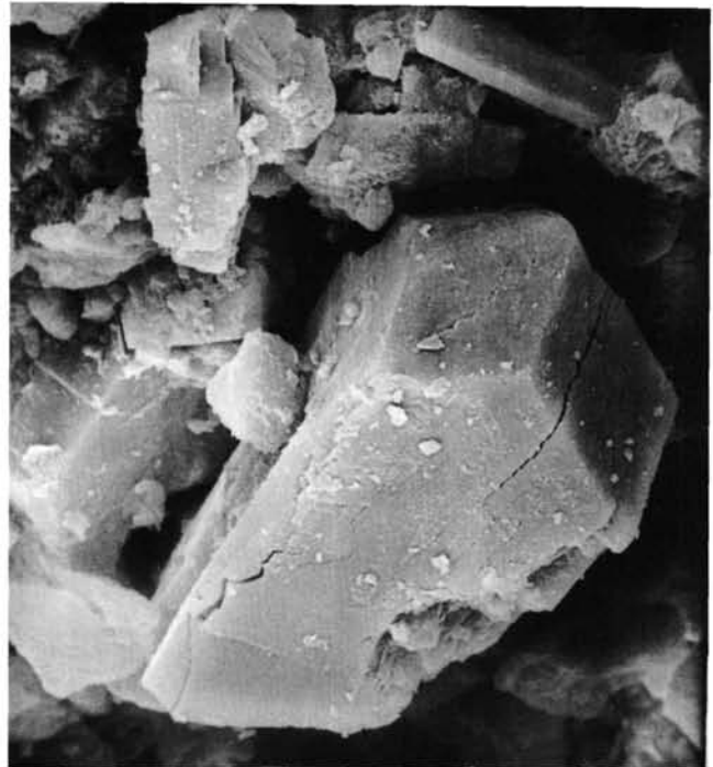
Figure 2. Roughly equant monoclinic phillipsite prisms in hemipelagic clay, Sample 382-15-3, 68-70 cm. SEM photograph.
