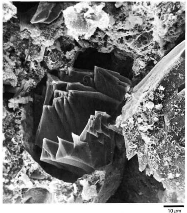
Figure 12. SEM micrograph of analcite crystals in volcaniclastic turbidites, Sample 386-13-3, 28-30 cm.
