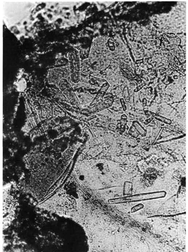
Figure 10. Petrographic micrograph of phillipsite laths in altered basaltic glass, Sample 386-5-2, 78 cm.
