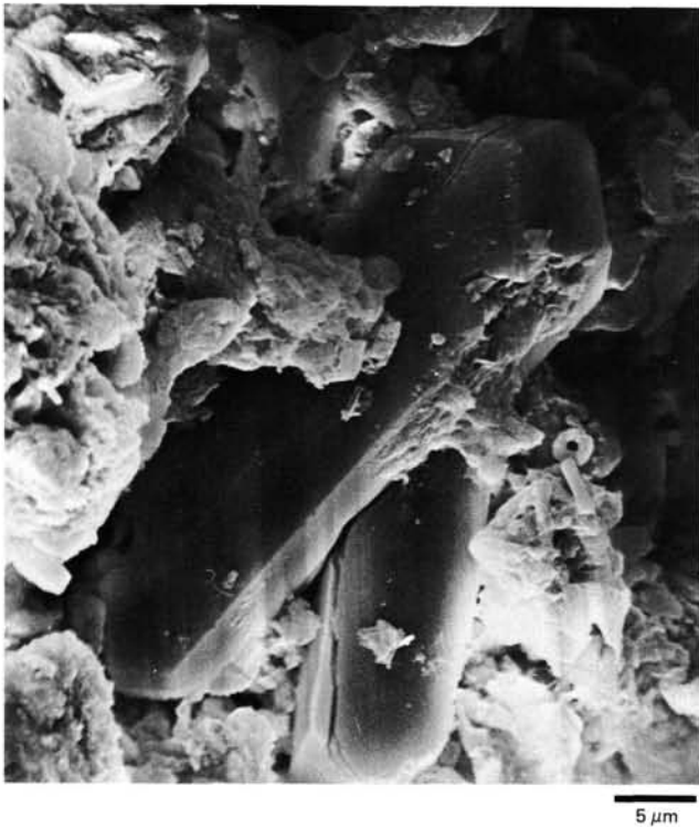
Figure 9. SEM micrograph of pseudo-orthorhombic phillipsite crystals in volcaniclastic turbidites, Sample 386-5-2, 78-80 cm.
