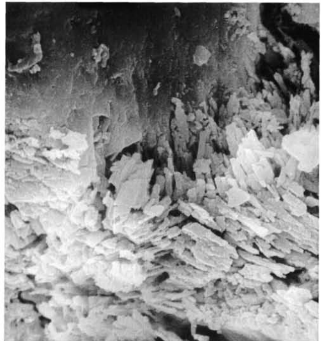
Figure 3. SEM micrograph of irregular clinoptilolite crystal in variegated clay, Sample 382-18-3, 68-70 cm.
