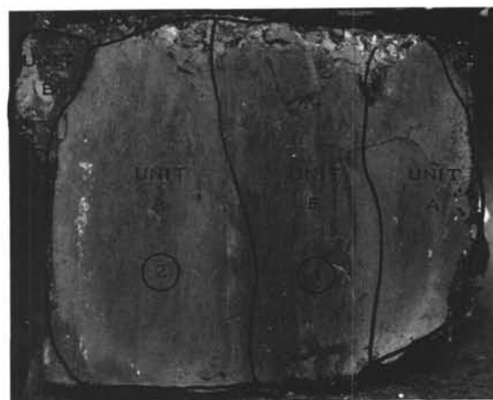
Figure 10. Site 368, Core 51, Section 2. Unit A—Clay, greenish-gray (5GY 4/1). Dark flecks appear to be plant macerals. Unit B—Clay, same as Unit A but dark yellowish-brown (10YR 4/2).
