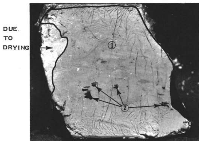
Figure 3. Site 368, Core 8, Section 3. Calcareous ooze, yellowish-gray (5Y 8/1). No fossils discernable. Clay clasts, olive-black (5Y 2/1).
