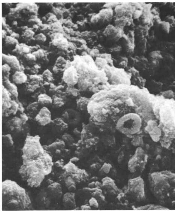
Figure 23. Site 288, 818.3 meters, Coniacian-Turonian, zeolite-rich claystone, porosity (818.4 m) 51%, scale bar 20 \mu ; sporadic nannofossils in a volcanogenic clay matrix.
