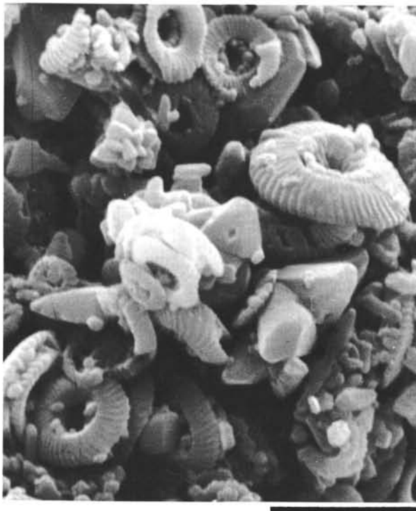
Figure 11. Site 288, 382.0 meters, late Oligocene, foram nanno chalk, porosity (382.7 m) 55%, scale bar 8 \mu ; coccoliths show corrosion and calcite precipitation; particles are welded together; large euhedral calcite crystals in the center (some having "negative crystals") are probably all overgrown fossil particles; radiating cluster of calcite crystals is the nannofossil Sphenolithus moriformis .
