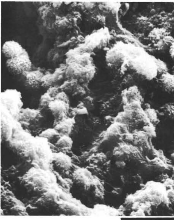
Figure 25. Site 288, 818.3 meters, Coniacian-Turonian, zeolite-rich claystone, porosity (818.4 m) 51%, scale bar 16 \mu ; imperfectly formed silica spherules.
