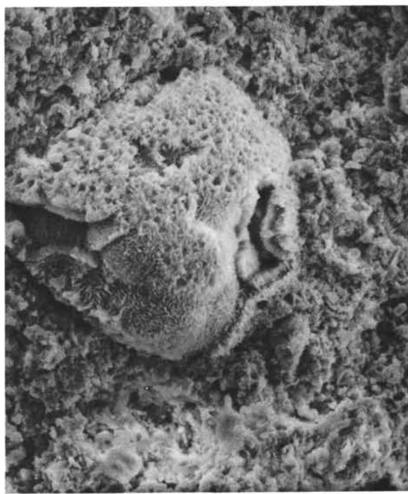
Figure 67. Site 289, 1084.2 meters, lower Eocene, siliceous limestone, porosity (1083.9 m) 11%, scale bar 30 \mu ; calcite substrate covered with a fine fibrous mineral, probably cristobalite; the same mineral is also present in the dense groundmass.
