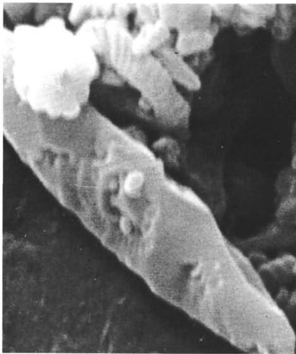
Figure 47. Site 289, 686.2 meters, late Oligocene, nannoforam chalk/ooze porosity (686.8 m) 51%, scale bar 6 \mu ; calcareous spicules as in Figure 46; note impression of coccolith in secondary calcite.
