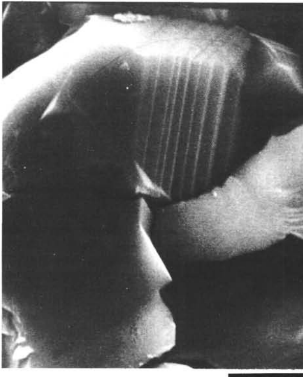
Figure 9. Site 288, detail of Figure 7, scale bar 6\mu ; interlocking quartz crystals in coarser crystalline patch of chert.
