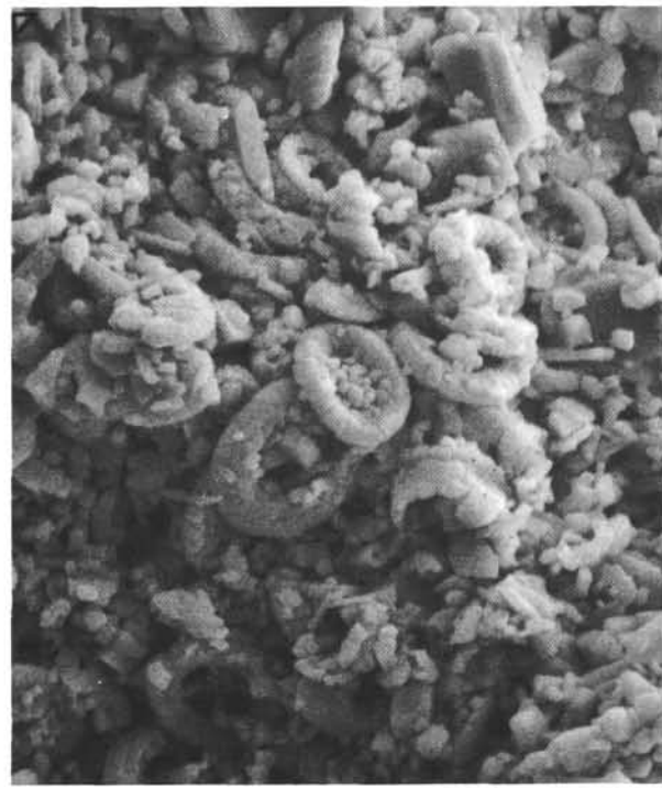
Figure 76. Site 289, 1175.3 meters, middle Maestrichtian, siliceous limestone, porosity (1175.3 m) 38%, scale bar 10 \mu ; micarb particles and relatively well preserved coccoliths; limited welding.
