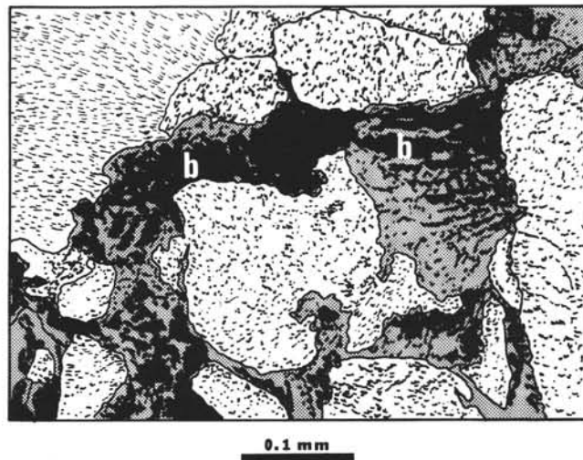
Figure 3. Biotite flakes (b) swollen and altered to mixtures of fine-grained clay and carbonate.
