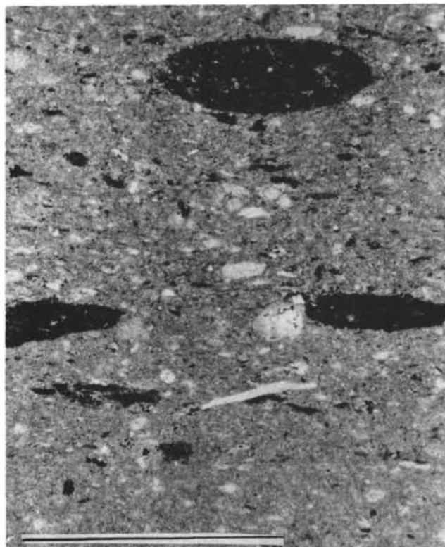
Figure 11. Burrowed limestone, with fish bone (lower center), recrystallized fossils, and flattened, highly organic burrows. Bar is 1 mm long. Turonian to Santonian. (146-36, CC).
