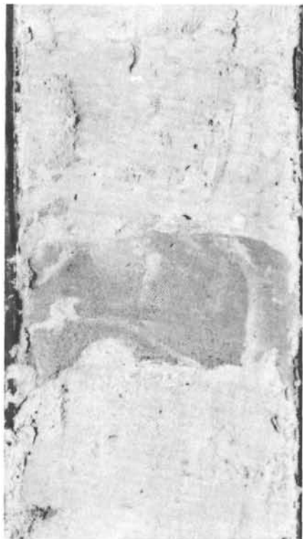
Figure 7. Radiolarian nannoplankton marl with distinct volcanic ash bed. Oligocene. (149-29-2, 113-125).
