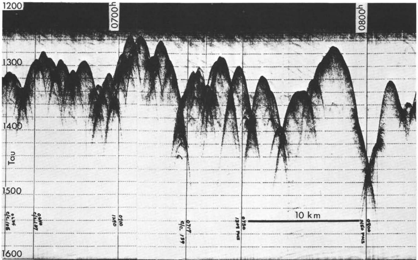
Figure 4. Echo-gram of the Mediterranean Ridge traverse during the Glomar Challenger site approach. The amplitude of the so-called "cobblestone" relief (Hersey, 1965 and Emery et al., 1966) progressively increases towards the south. Site 130 was located in a regionally smooth, low-lying area where sub-bottom stratification could be observed in reflection profiles.
