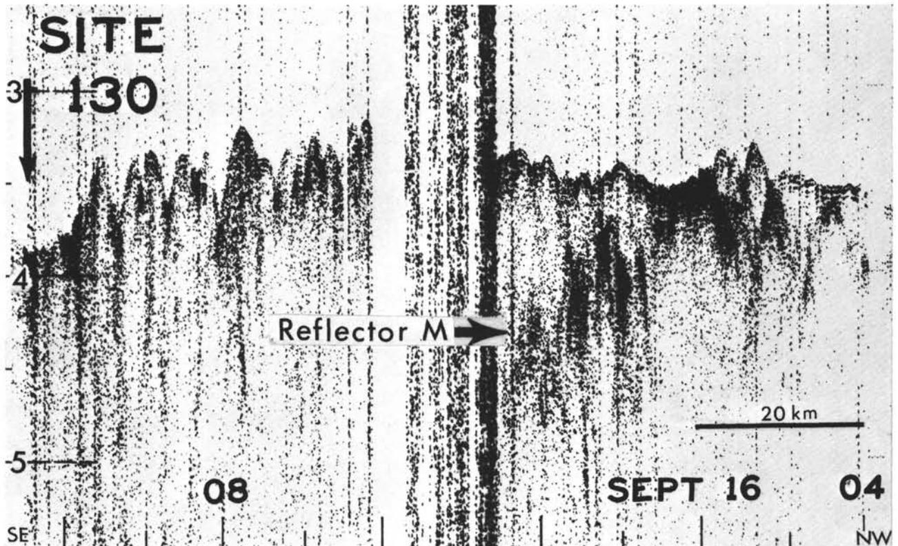
Figure 3. Seismic reflection profile of the *Glomar Challenger* showing a crossing of the Mediterranean Ridge while proceeding to Site 130. Note the descent of Reflector M towards the southeast and an increase in the amplitude and wave length of the surface relief. Vertical scale is in two-way reflection time (seconds). Vertical exaggeration is  $\approx 28:1$ .
