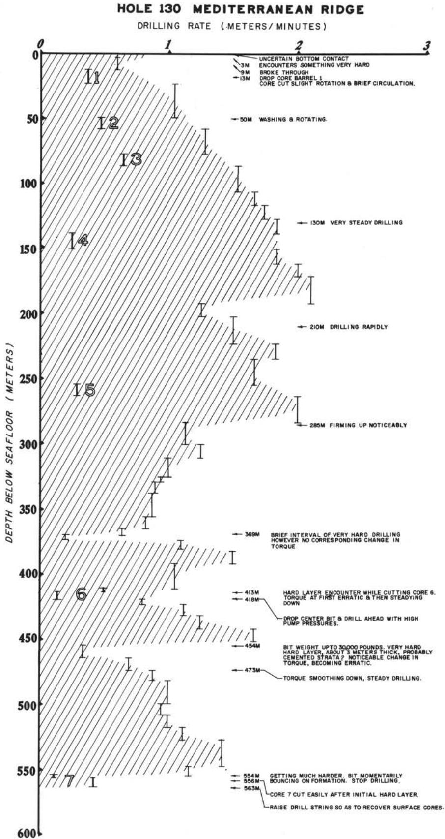
Figure 6. Penetration rates during the drilling of Hole 130.
