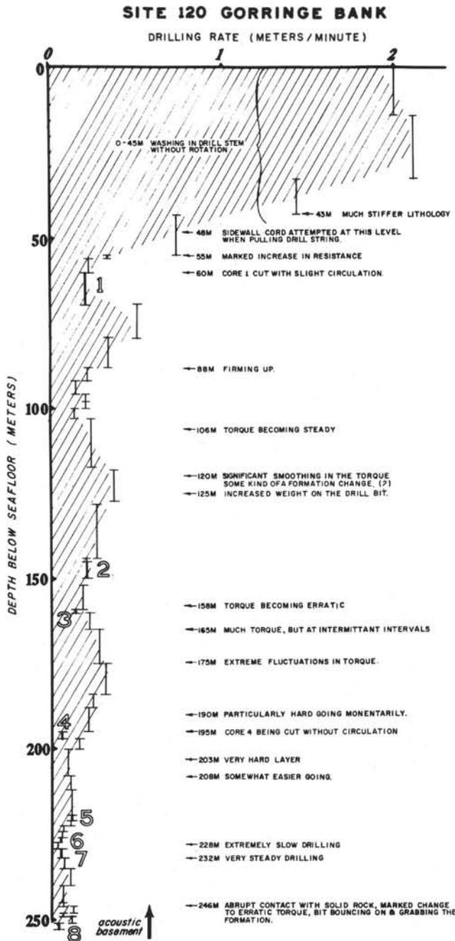
Figure 4. Drilling rates versus subbottom depth for Hole 120. Bars show average rates of penetration for various intervals of uniform drilling. Intervals of coring are not included in the fitted curve, since they were cut often without circulation and with lesser bit pressures on the formation. Note the basement contact at 246 meters and a major change in formation hardness at 55 meters.
