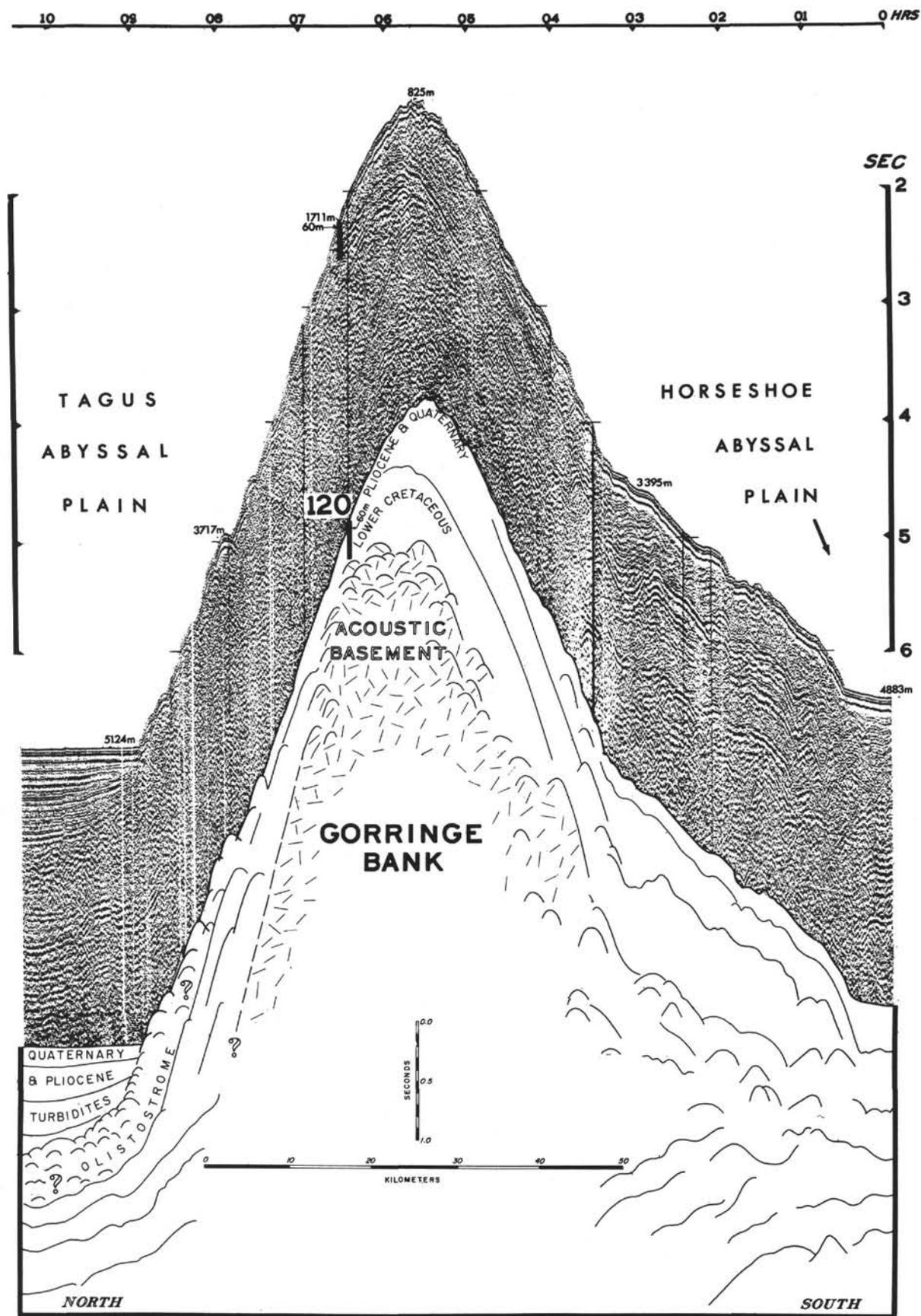
Figure 2. Seismic reflection profile (Flexotir) across the Tagus Abyssal Plain, Gorringer, Bank, and the Horseshoe Abyssal Plain. Vertical scale is in seconds of two-way travel time. The profile, made by the R/V Jean Charcot, was given to us by X. Le Pichon.
